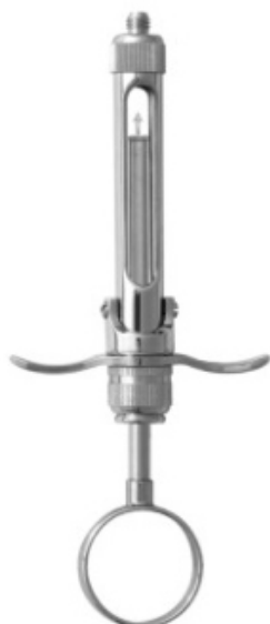
S-0700-22 Cartridge Syringe Cylinder with Aspiration, Metric /Us threads. Non folding- chromium Plated brass. 1.8 CC & 2.2 CC
